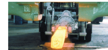
Performing-3ton Air Drop Hammer
